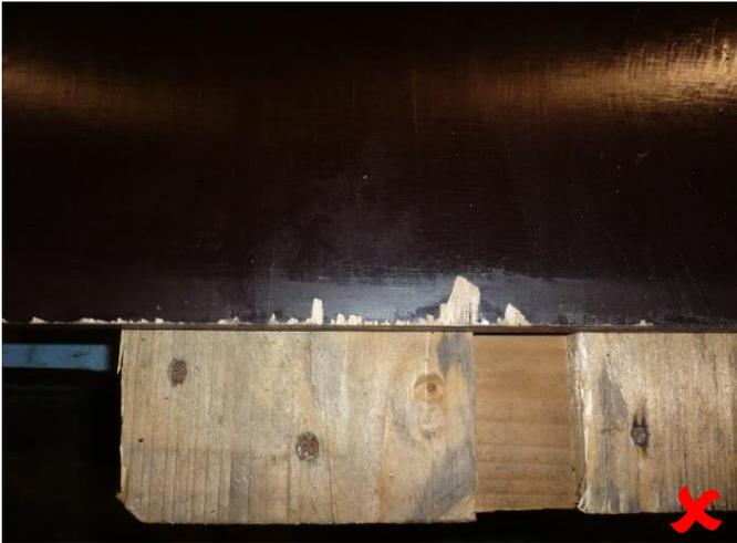
Image 6. Incorrect machining due to lack of support.
