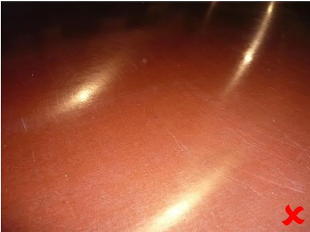
Image 3. Marks on the panel surface due to improper handling.
