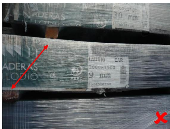
Image 2. Wood battens should be aligned
