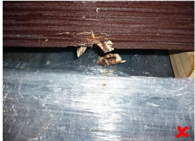
Image 4. Panel damaged by Forklift hit.
